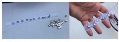
Easy taping method: Line up batteries, apply a strip of tape to them, flip them over, and put another piece of tape on top.
