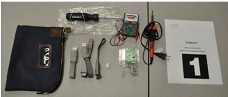
Skimmer, card reader/writer, screwdriver, voltage meter to test the connection when making the skimmer, and soldering gun to connect everything.
